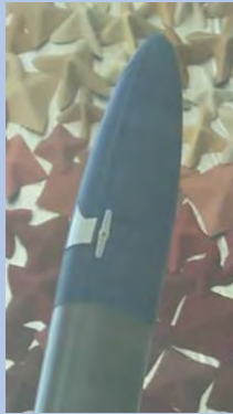
Stage 1: Door and parachute held in position by the servo. Detecting for apogee.
