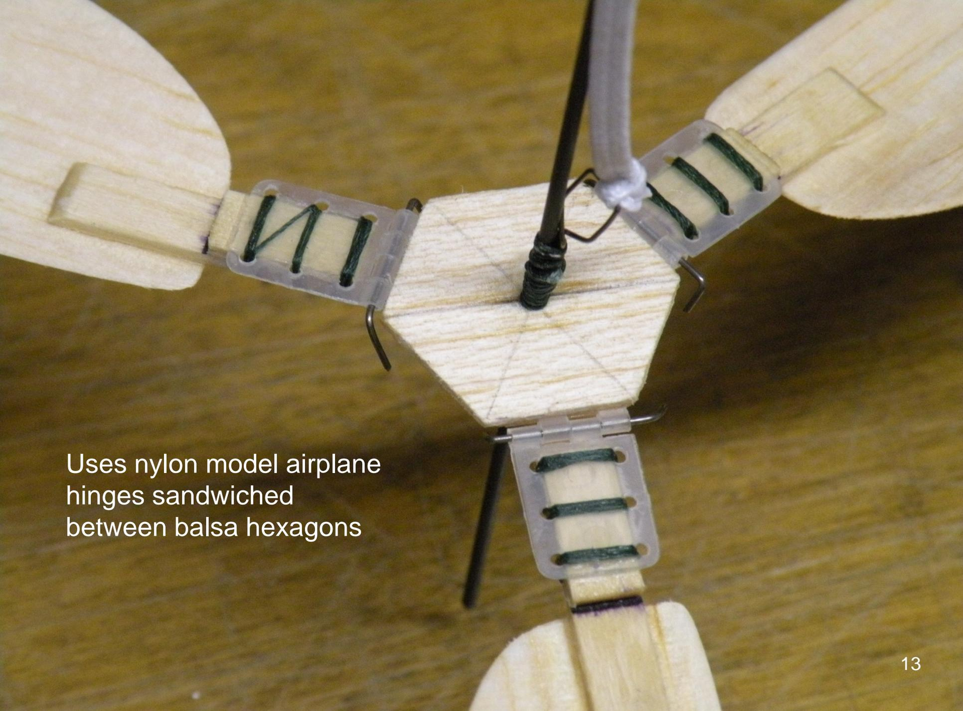
Uses nylon model airplane hinges sandwiched between balsa hexagons
