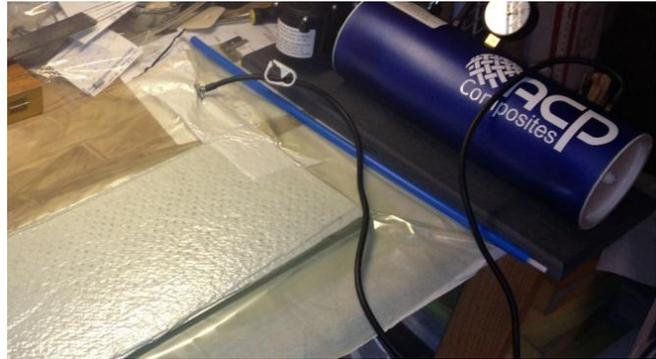
This document assumes that vacuum bagging will be done using the ACP bag tube and clip supplies. However, a layup (w/o tissue) can be performed at ambient pressure, although the resulting laminate might be somewhat heavier due to excess resin. Tissue will tend to absorb resin and may wrinkle if the laminate isn't under pressure.
