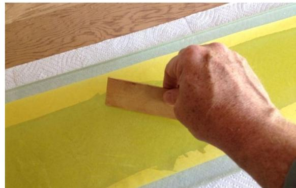
The final step is to use the spreader tool as a squeegee to remove any excess epoxy from the laminate. Remember that the strength of the laminate comes from the plies, so excess epoxy only adds unnecessary weight. You'll quickly get a feel for how much pressure to apply to remove excess resin.
