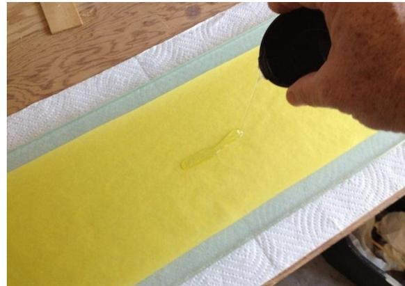
If there are additional layers of the laminate, carefully place the next ply onto the wetted-out first ply. Apply more epoxy, and spread the epoxy to wet out the additional ply. Repeat this process until all of the plies are done.
