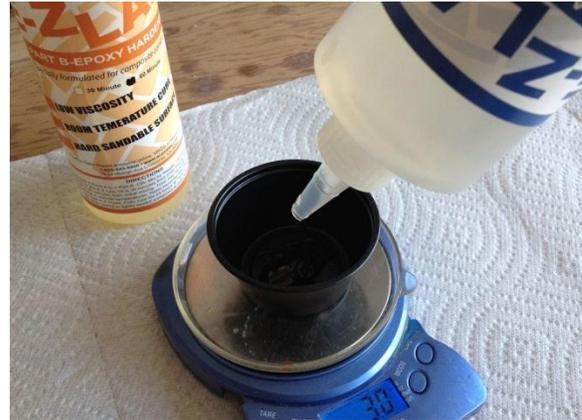
Be sure to accurately measure the resin and hardener amounts. Using a scale accurate to 0.1 grams is recommended. After pouring the resin and hardener, be sure to stir very thoroughly.
