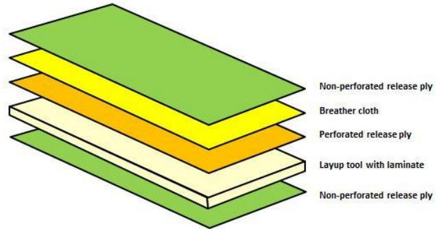
The perforated release ply allows any excess resin to bleed out of the laminate and into the breather cloth. The top and bottom layers of non-perforated release ply prevent the assembly from bonding to the vacuum bag. You can use some masking tape to keep the "sandwich" assembled.
