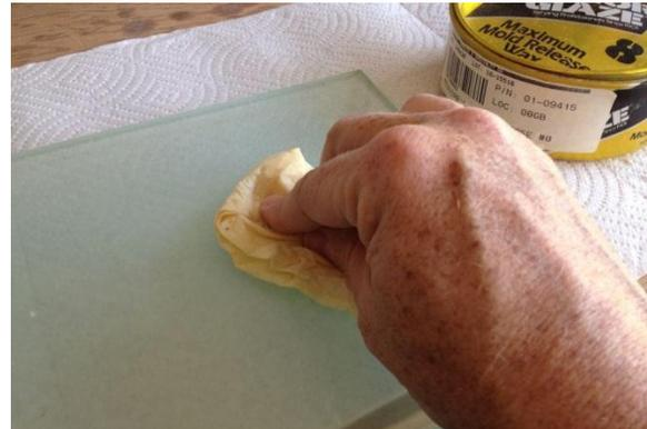
The layer of wax might be sufficient release treatment. However, to be prudent, apply a layer of release agent. Spray-on release (such as LPS MRX silicone mold release<sup>7</sup>) provides a smooth uniform finish. Liquid release (such as FibRelease<sup>8</sup>) might also be used. If using liquid release, allow the release material to dry before proceeding with the layup.
