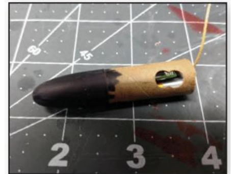
Figure 2. Adrel ALT-BMP now fully installed in the nose cone with extended shoulder.
