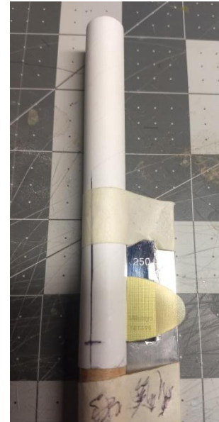
Figure 3 the 1st fin is put in position on the fin jig for attachment.
