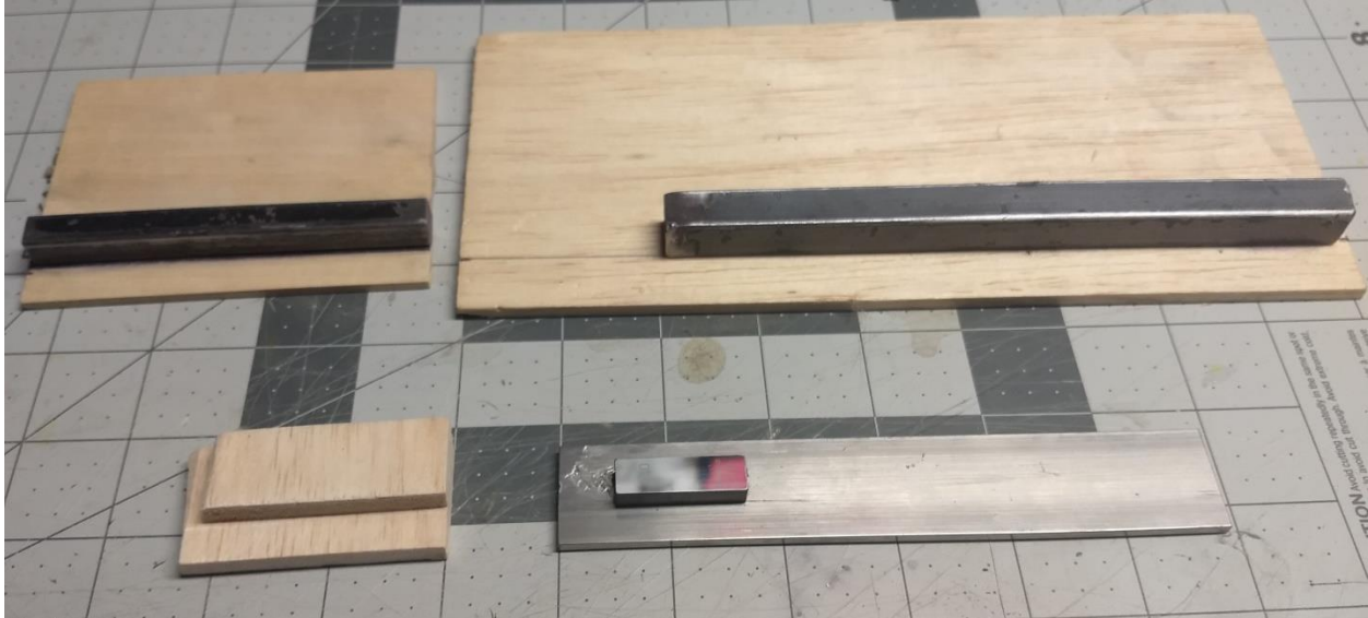
Figure 1 The author's assortment of fin jigs through the years made with balsa, steel, and stainless steel and for different body tube sizes from 13mm to 24 mm.
