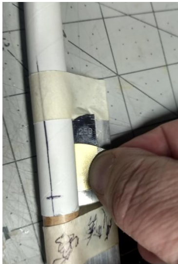
Figure 4 Fin held in place to stay flat against the body tube. The CA is put in the fin joint with the other hand.
