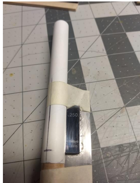
Figure 2 The body tube is secured to the fin jig with tape.
