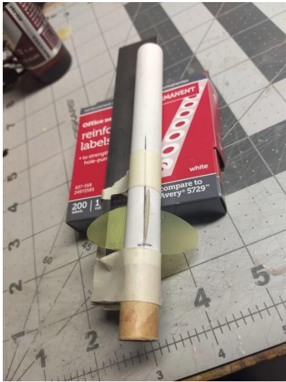
Figure 4 Attachment of 3rd fin. Note fin jig is raised so the "bottom" fin has room to extend below jig.
