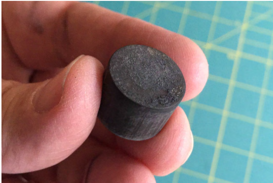
Figure 7.4-2. The piston floating head cap did not show any significant charring or melting.
