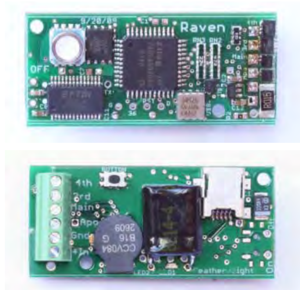
Figure 6.1-1. The Raven 3 altimeter includes an axial accelerometer that measures \pm 70G at a 400 Hz sampling rate.
