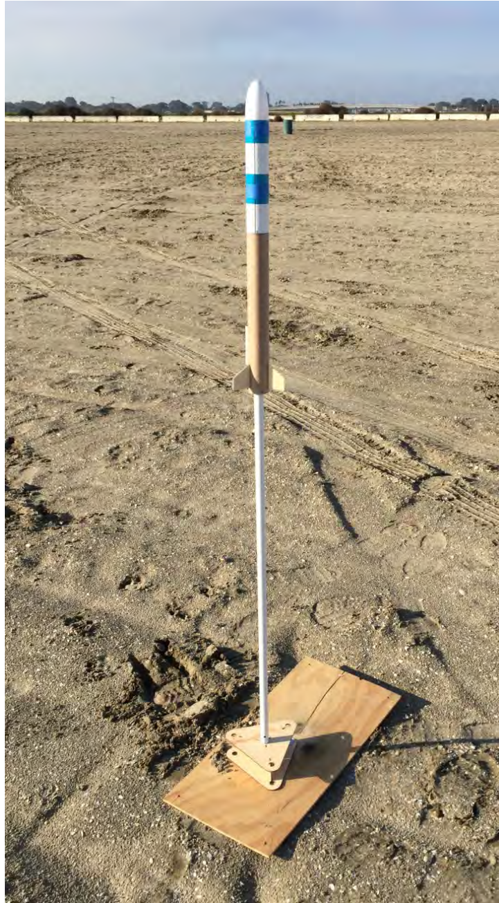
Figure 6.3-1. The piston test model was attached to the piston launcher without lateral supports.
