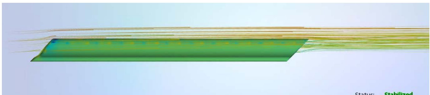
Sim #28 - 1/8" X 2" long launch lug with glue fillets, radiused LE, and Swept LE and TE - air flow streamlines.
