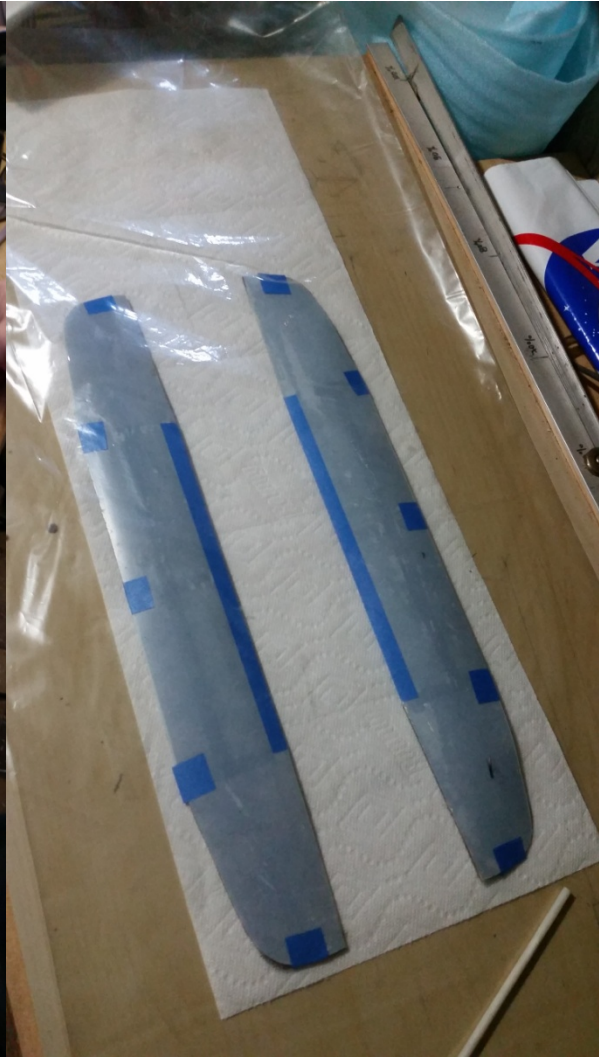
Picture12- Place cores into a vacuum bag
