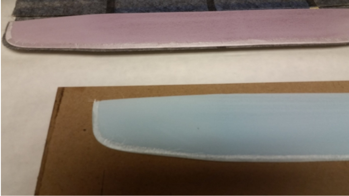
Picture6- Covering front edge with glass fabric
