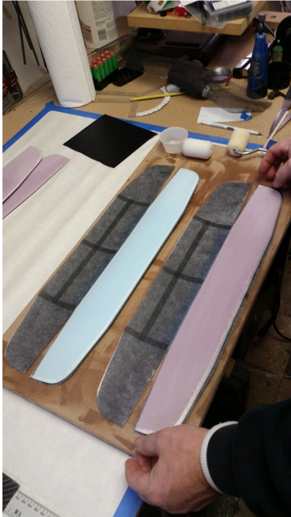
Picture11- Place top and bottom Mylars on a core and line them up
