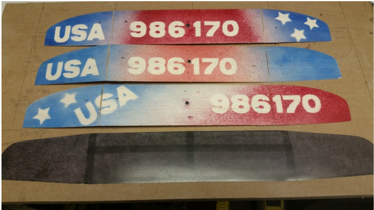
Picture13- Picture of laminated wing after about 24 hours in vacuum bag
