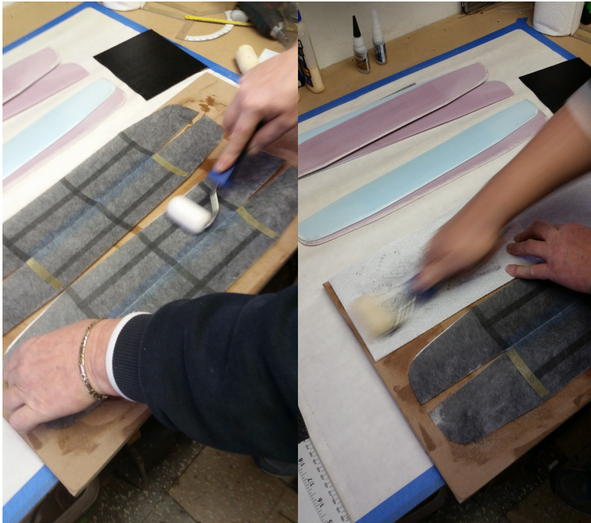
Picture9- Appling epoxi on shell
