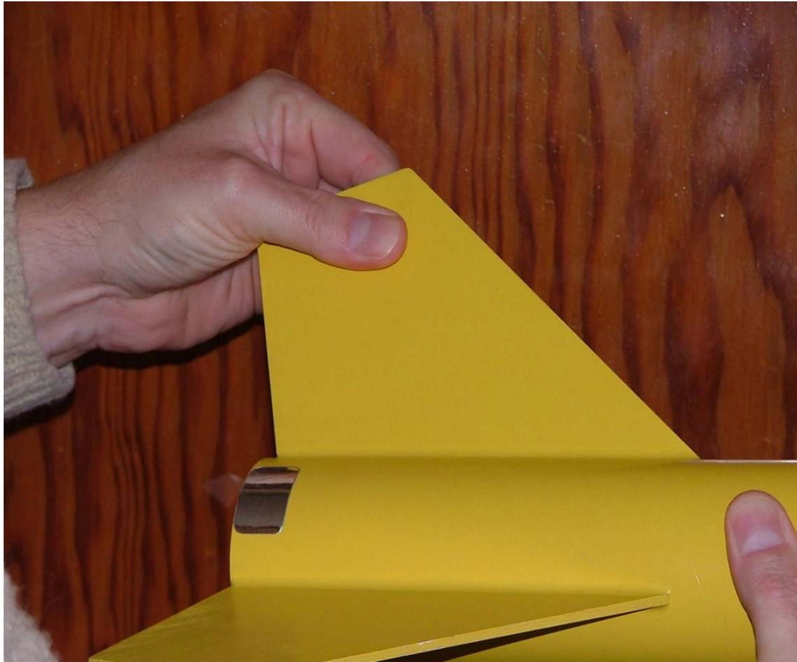
Are the fins secure? Are they straight? Are the fillets intact?
