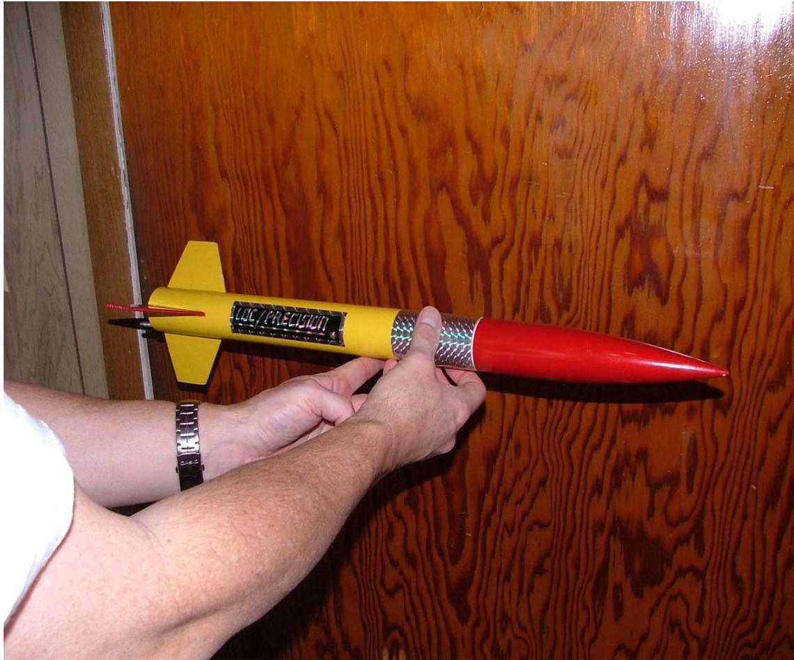
Is the model stable? Check that CG is well ahead of fin leading edge. 32
