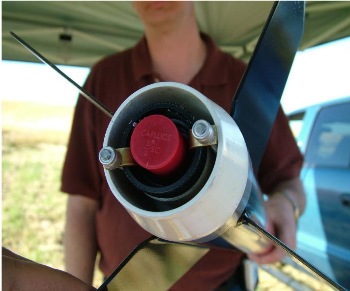
Is the motor secure? Will it “fly through” the model or pop out at ejection? 31
