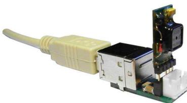
Adapter has a built-in complete control system of battery recharge (single-cell Li-Pol).
