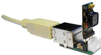
cable for connecting the altimeter yourself. To do this in a typical USB cables cut off one plug (leave the plug connected to a computer) and isolate the wire length of approximately 1.5 cm. Then color-coded wires as in the photo should be soldered (or tightened) to the appropriate connector pins. Please note that the pin spacing is 2mm. Below are listed the addresses of shops and types of connectors needed
