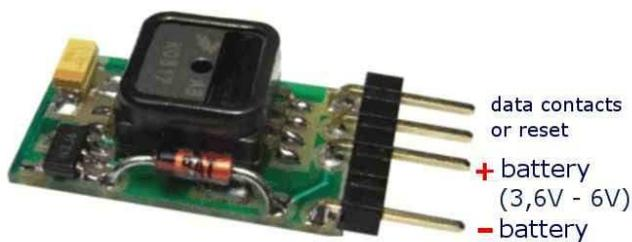
are addresses of online shops where you can buy these connectors, and the names of these connectors. The figure shows the power connection. Altimeter is protected against reverse connection of power supply.
