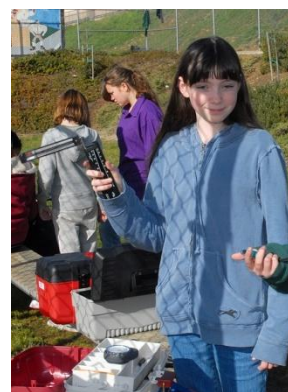
Figure 7 A meteorologist operates the sling psychrometer
