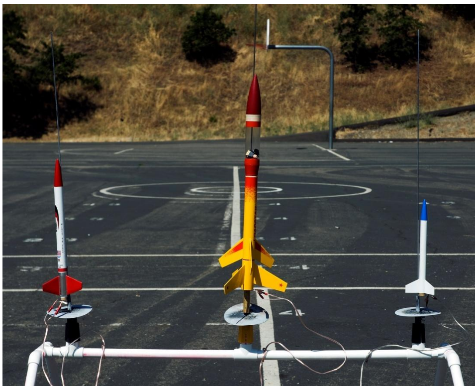
Figure 11 a PVC launch pad for 3 rockets made by the author. The rockets from left to right are the Apogee Avion, the Estes Loadstar, and a scratch built Paradigm 5.
