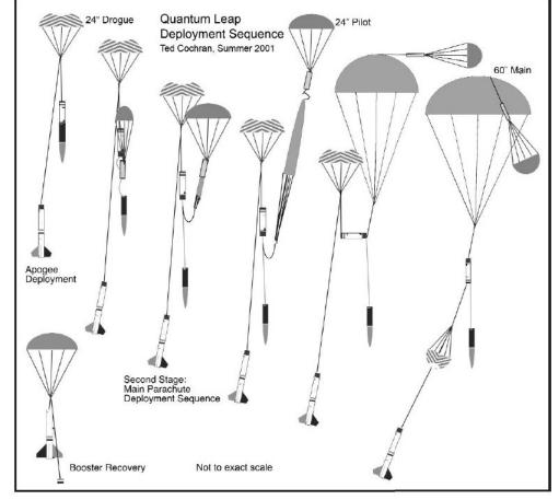
slightly marred by an early deployment of the drogue—caused by the motor-which led to early main deployment and a 3" zipper of the main chute section. There is a lesson here: Motor ejection is a good for redundancy, but is not without failure modes of its own (none of which is as bad as a ballistic descent, however).
